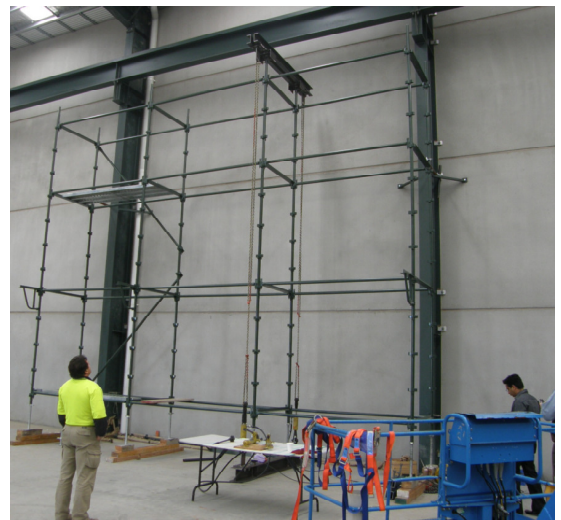
FIG.1. SCAFFOLD TEST ASSEMBLY
