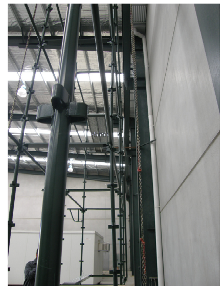
FIG.4. DEFLECTION IN STANDARDS FROM TEST LOADING
