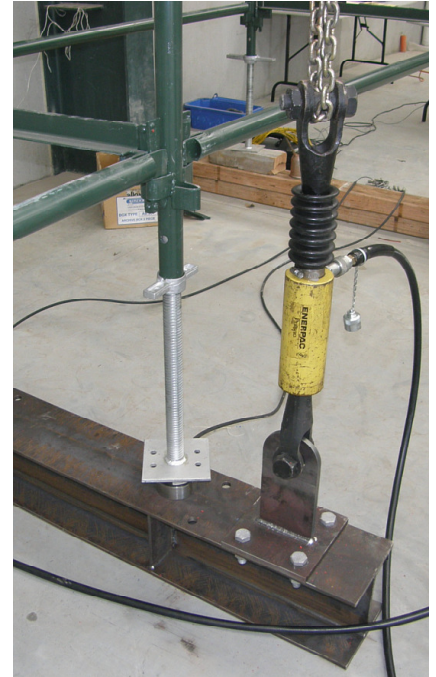
FIG.3. LOADING & FORCE DEVICE
